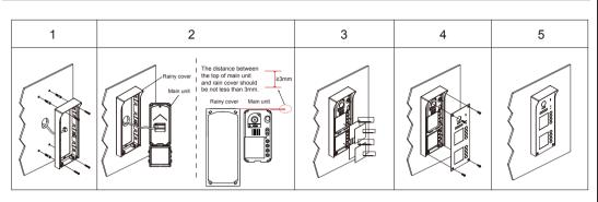
1. Drill holes in the wall to match the size of screw stoppers, then attach the rainy cover to the wall.
