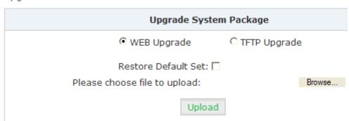
Check "WEB Upgrade" radio button and click "Browse" button to locate the new firmware in your PC hard drive. Click "Upload" it will ask you to confirm if restart the IP PBX system to complete the upgrading process. You can click "Yes" to continue upgrading.
