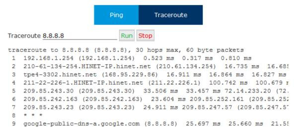
After the process system will notice "Trace Complete" and you can see which routes the packets taken before reaching the final destination.
