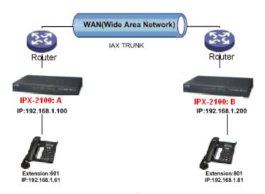
**Step1:** Configure the mapping rule of IPX-2100-A on the router.
