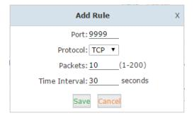
In this case, it will block the IP which will send more than 10 packets to the port 9999 within 30 seconds, this rule will prevent brute-force attempts of the web login.
