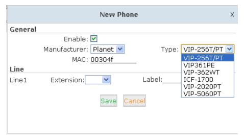
Enable Phone Provisioning in [Basic], select the IP Phone manufacture, input MAC of the phone, and select the extension for provisioning.
