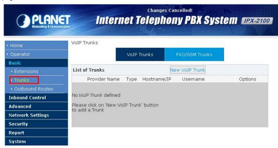
Planet IP PBX supports 3 kinds of trunks: VoIP Trunks, FXO Trunks and GSM Trunk.
