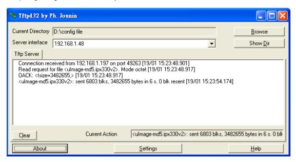
Please click "Browse" on the TFTP application window to locate the new firmware. And in the "Server Interface" dropdown list it's a list of your PC network interfaces. Please select a correct interface (in the same network) which can access the IP PBX system.
