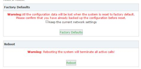
As you can see here on this page, you are able to reset and reboot the IPPBX system directly via web GUI.
