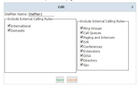
The calling rules in the left column are for external calls and calling rules in the right column are for internal calling. If you want to restrict some uses from calling out through some trunk lines or you don't want them be able to call some internal destinations, you can create new dial plan by clicking the "New DialPlan" button.
