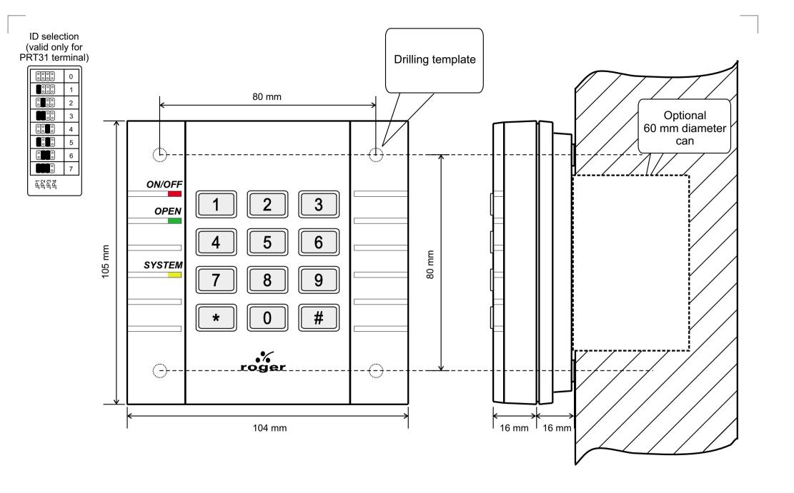
The front and side view of PR301 controller and PRT31 terminal. Scale 1:1
