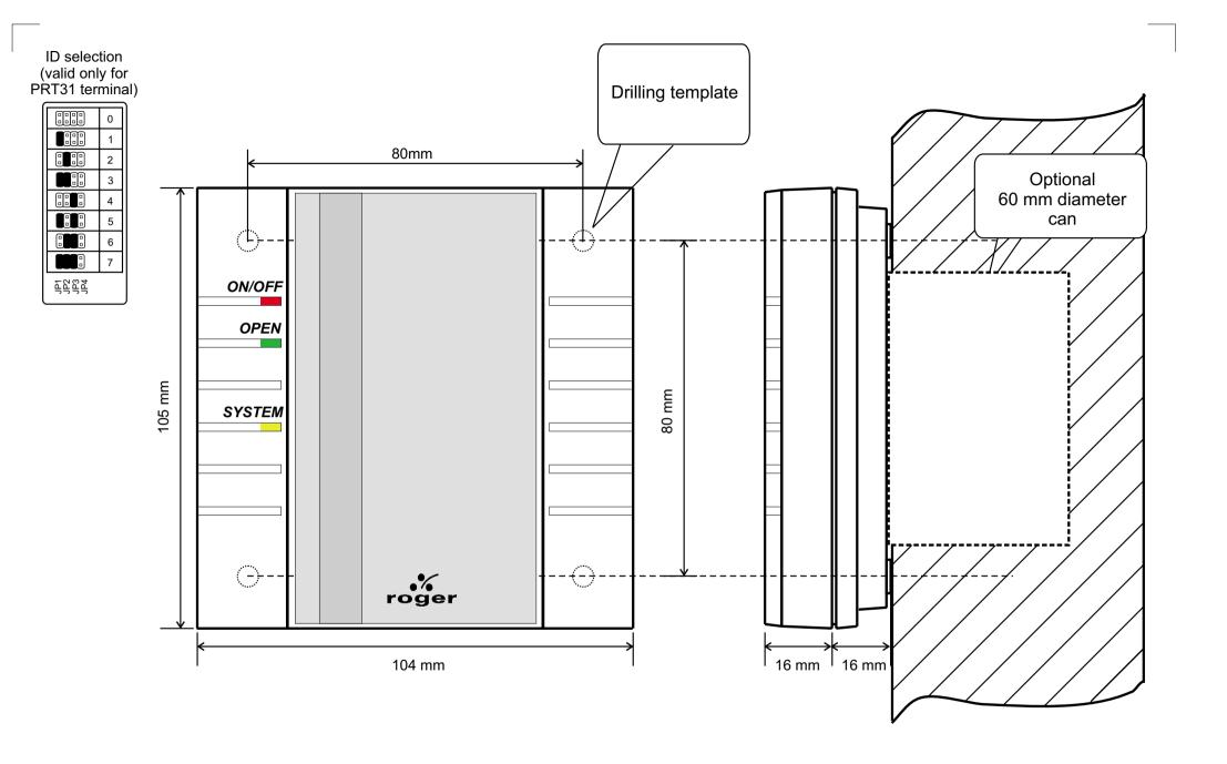
The front and side view of PR201 controller and PRT21 terminal. Scale 1:1
