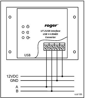
Fig.1 Connection UT-USB to RACS system
