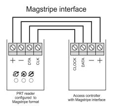
When employing **Magstripe** transmission format, data is transferred to the host using electric signal waves transmitted over the CLK and DTA lines. In **Magstripe** format a dual color LED STATUS ilights steady in red, LED OPEN is controlled by IN1 while buzzer is controlled by IN2. Both inputs (IN1 and IN2) are triggered by supply minus. In addition, whenever card is read or PIN is entered reader activates momentary LED SYSTEM and buzzer. Card code is always transmitted as a whole number
