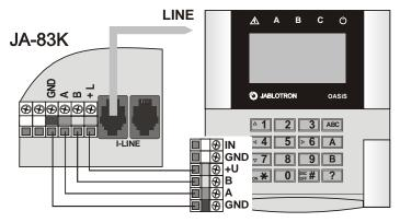
fig. 1 Connection with the control panel
