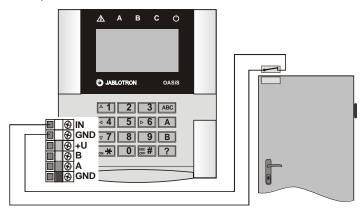
fig. 2 An example of door detector wiring
