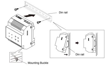
Step1: Mount the din rail to the wall with screws ;
