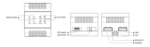
**DIP:**DIP switches,DIP settings refer to 3.
