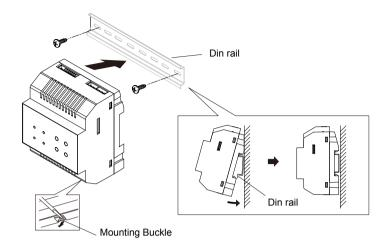
Step1: Mount the din rail to the wall with screws;
