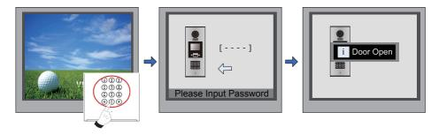
When the Door Station is in standby, Press "#"
