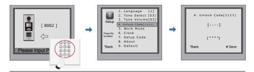
Press "#",Input "8002", then input Setup Code or Admin Code(88888888 or 66666666 by default) Press "4" to enter unlock code item.
