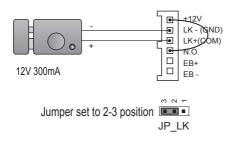
set to Normally open on the Unlock Relay mode
