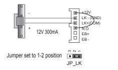
set to Normally Closed on the Unlock Relay mode
